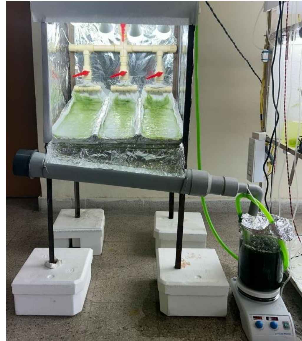
Fig. Lab Scale Incline Microalgal Biofilm Bioreactor (IMBB)
