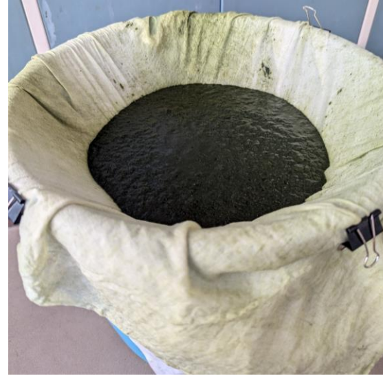
Fig. Filtration of algal biomass
