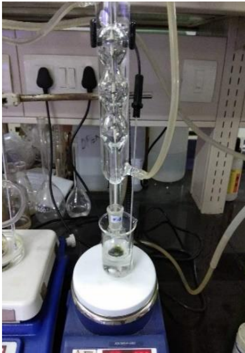
Fig.: 2-step transesterification ( \text{H}_2\text{SO}_4 & \text{NaOH} ) at 70 °C for 3h
