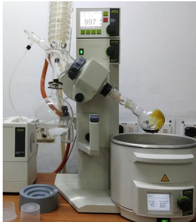
Fig.: Solvent separation (n-Hexane) in rotary evaporator
