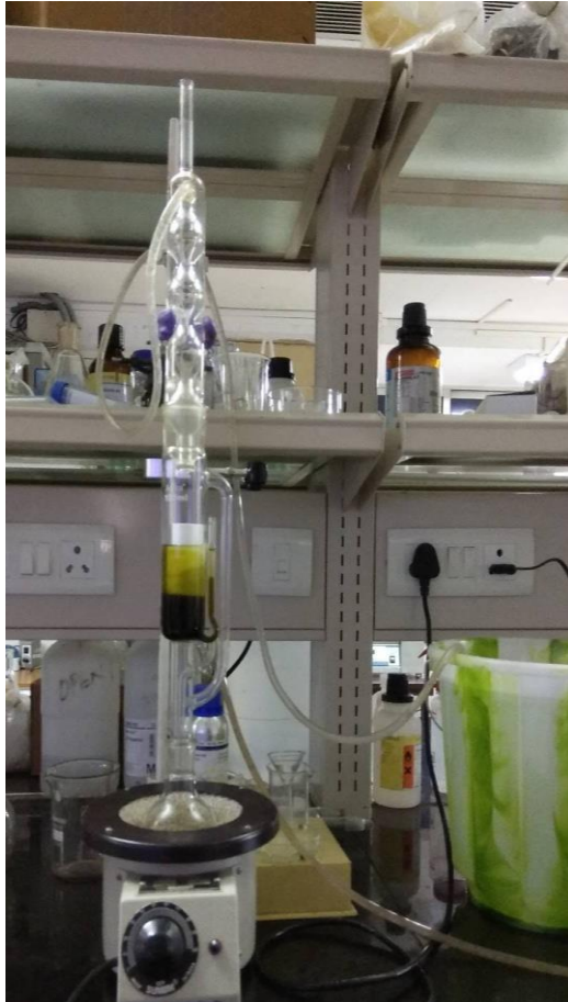
Fig.: Lipid Extraction in a Soxhlet apparatus
