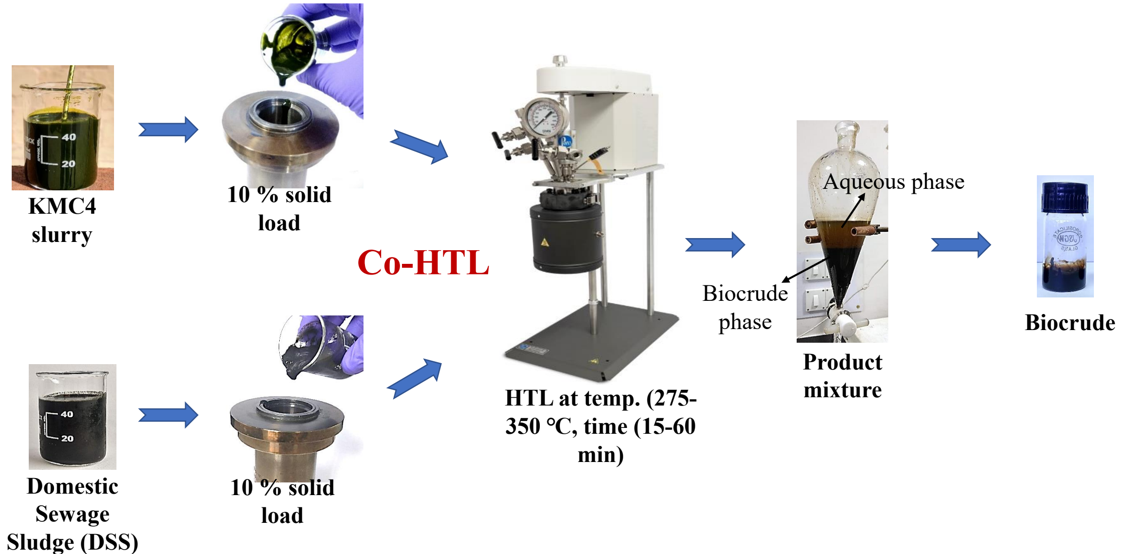
Fig.: Schematic of HTL/Co-HTL experimental process
